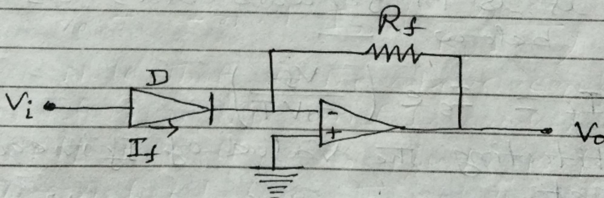
In the circuit above, the non-inverting input terminal of the OP-amp is connected to ground. It means zero volts is applied to its non-inverting input terminal.
